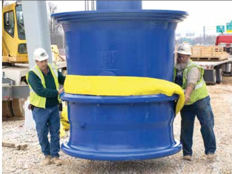
Image 2. The largest submersible propeller pumps produced by the project's pump manufacturer.
